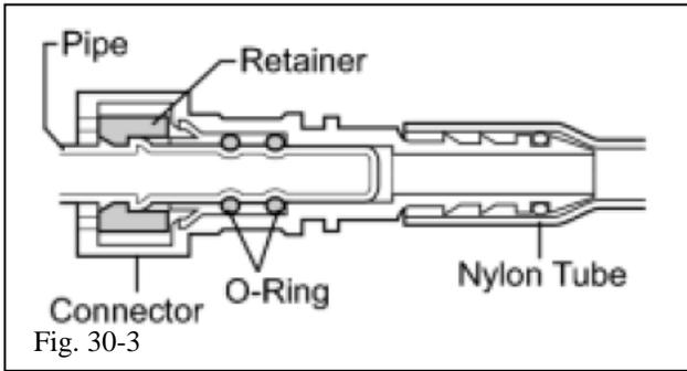
(2) Pinch and pull the main tube connector to disconnect it from the pipe (Fig. 30-3).
