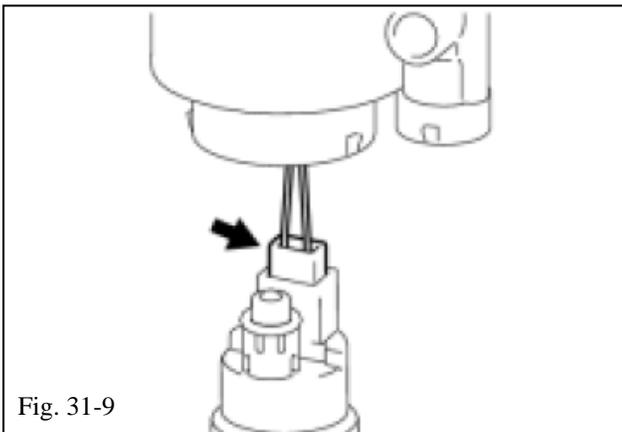
(i) Disconnect the fuel pump harness from the fuel pump (Fig. 31-9).
