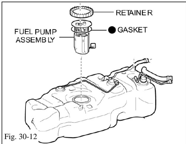
(q) Remove the fuel pump assembly from the fuel tank (Fig. 30-12).
