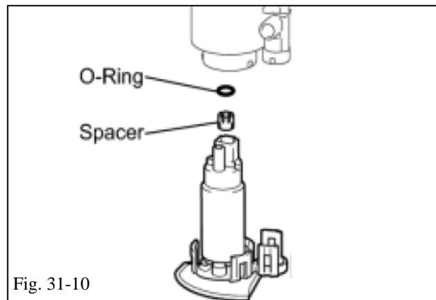
(j) Remove the fuel pump discharge O-ring and spacer from the fuel pump (Fig. 31-10).
