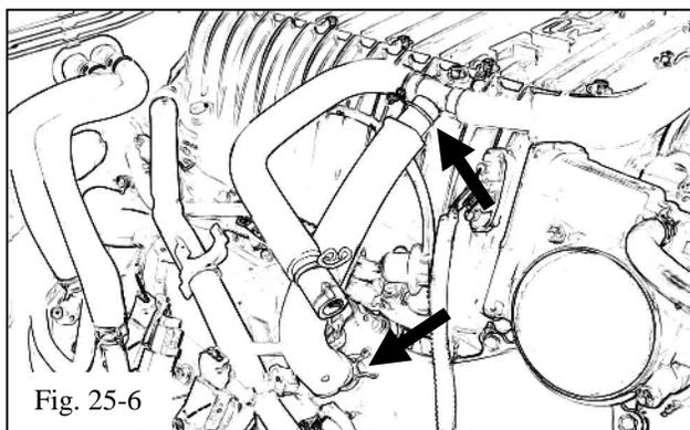
(d) Remove the middle hose from the "T" and trim it so that it will neatly fit between the "T" and the RH cam cover.
