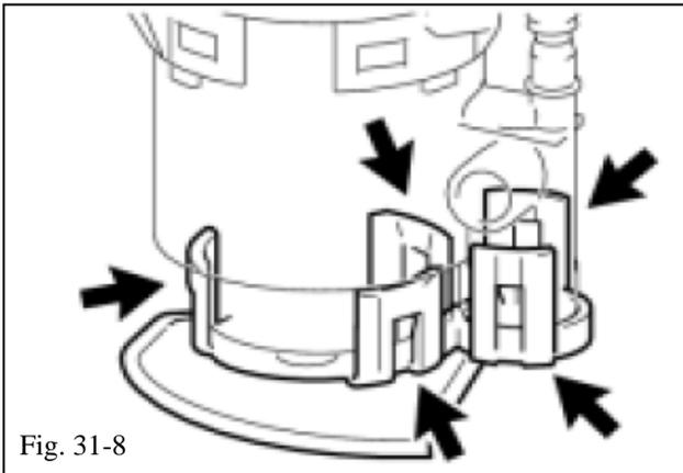
(h) Use a small screwdriver to detach the 5 claws from the claw holes and disconnect the fuel pump from the suction plate with filter (Fig. 31-8).
