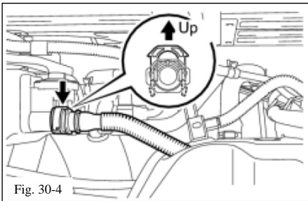
(e) Pull up on the retainer clip to disconnect the vent line hose (Fig. 30-4).
