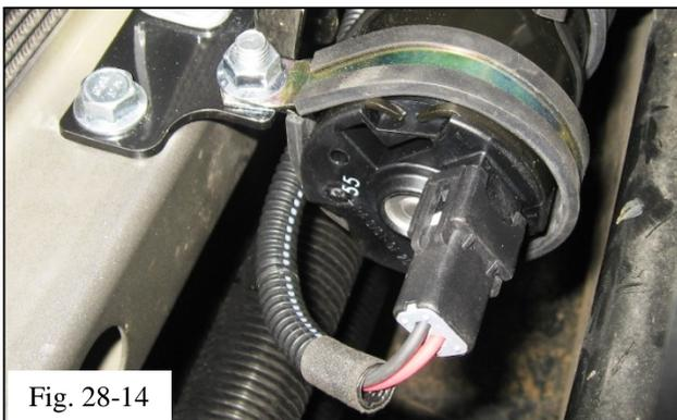
(m) Plug the electrical connector into the pump (Fig. 28-14).
