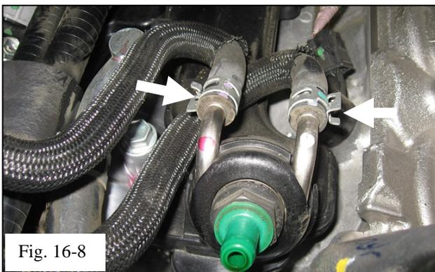
(l) Make certain the hose clamps on the water bypass hoses No. 9 & No. 10 are oriented as shown in Fig. 16-8.
