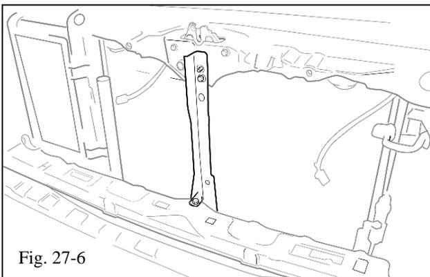
(f) Remove the radiator support brace by removing the 2 bolts (Fig. 27-6). Retain the brace and the bolts for reuse.
