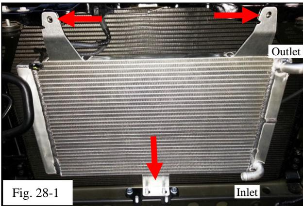
(a) Set the intercooler low temperature radiator (LTR, Item #1) in front of the A/C condenser (Fig. 28-1).
