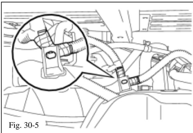
(f) Disconnect the wire harness from the fuel tank (Fig. 30-5).
