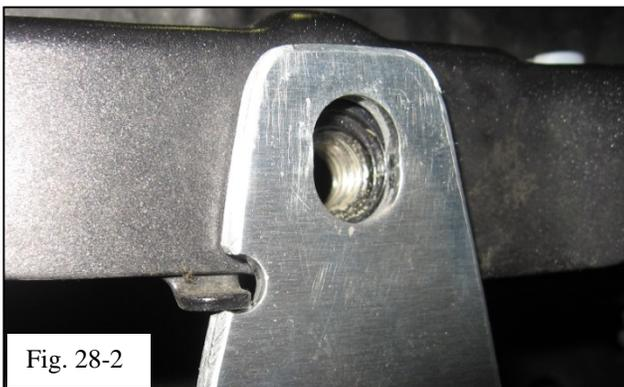
(1) Align the upper mounting tabs with the horn mounting holes (top, Fig. 28-1 & Fig. 28-2).
