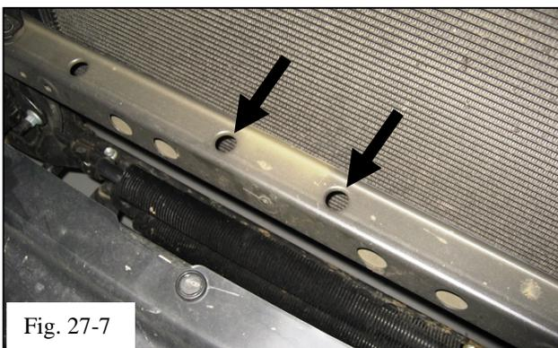
(g) With the radiator support brace removed, two large stamped holes are visible (Fig. 27-7). They will be used to attach the intercooler pump mount.
