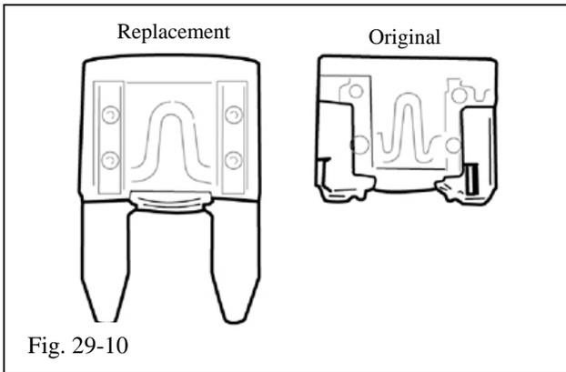
(h) The original (removed) fuse and the new replacement fuse (Item A3) are shown in Fig. 29-10).
