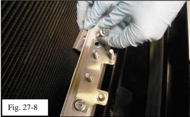
(h) Mount the intercooler pump bracket (Item A4) to the lower radiator support with 2 rectangular body nuts (Item A6) and 2 M8 nuts (Item A5) (Fig. 27-8). Leave the bolts finger tight for now.
