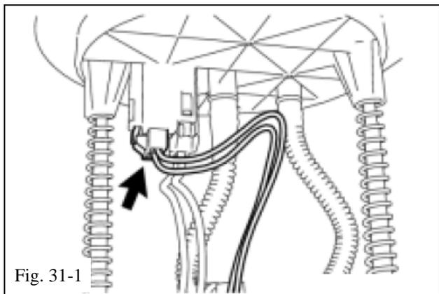
(a) Disconnect the fuel sender gauge connector (Fig. 31-1).
