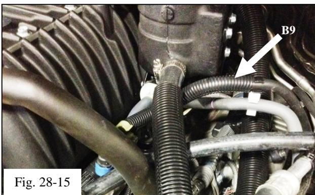
(n) Place the 1/2" X 6" split loom (Item B9) over the fuel line (Fig. 28-15).
