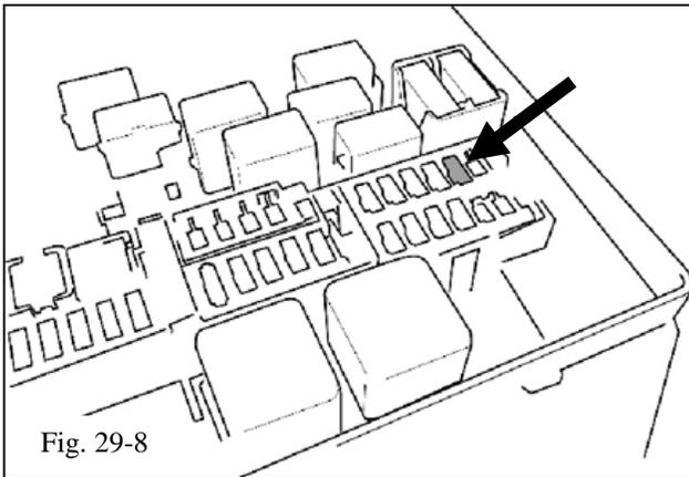
(g) Remove the 10 amp ignition fuse (Fig. 29-8 & Fig. 29-9).
