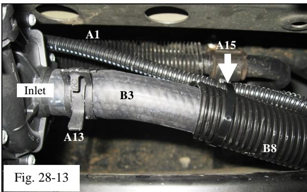
(l) Secure the pump wire harness (Item A1) to the coolant hose assembly with a tie wrap (Item A15) (Fig. 28-13).
