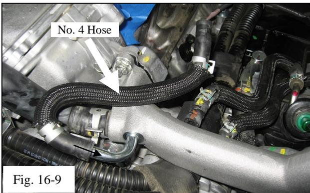
(m) Install the No. 4 water bypass hose (Fig. 16-9). This hose was removed in Step 12(c).
