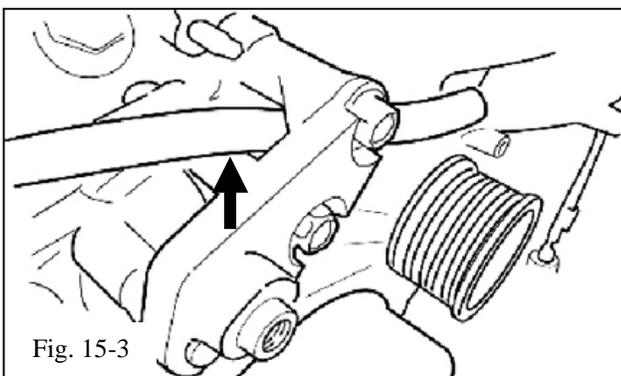
**NOTE: Fig. 15-3 does not show the mesh sleeve on the No. 6 water bypass hose. Make sure the mesh sleeve extends down between the legs of the bracket.**
