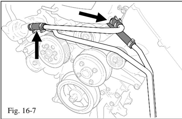
(k) Slide a supplied screw clamp (Item C3) on each end of the “J” shaped bypass manifold (Item C2) and attach it to the thermostat housing and the coolant crossover manifold (Fig. 16-7). Ensure the tube fits comfortably without any kinks and tighten the screw clamps.
